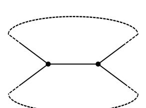
For identical frequencies, if no pair of vertices of degree larger or equal to 3 are connecected by a single edge, then all the stable fixed point have all angle differences in  $[-\pi/2, \pi/2]$  and thus  $\mathcal{N} = \mathcal{N}^*$ . The right-hand-side of Eq. (8) is then a bound on the total number of stable fixed points [2, 6].
