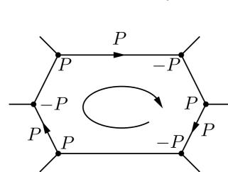
As the angle differences along the edges of the network are taken modulo  $2\pi$  in the interval  $(-\pi, \pi]$ , the sum of angle differences around a cycle is an integer multiple of  $2\pi$ ,
